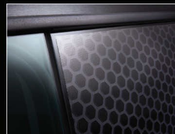
▲ Create a uniform relief cut between window graphic and rubber molding.
